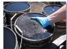
**Carbon is inert, non-toxic, non-degrading, and traps virtually all organics, whether in vapor or aqueous phase.**
